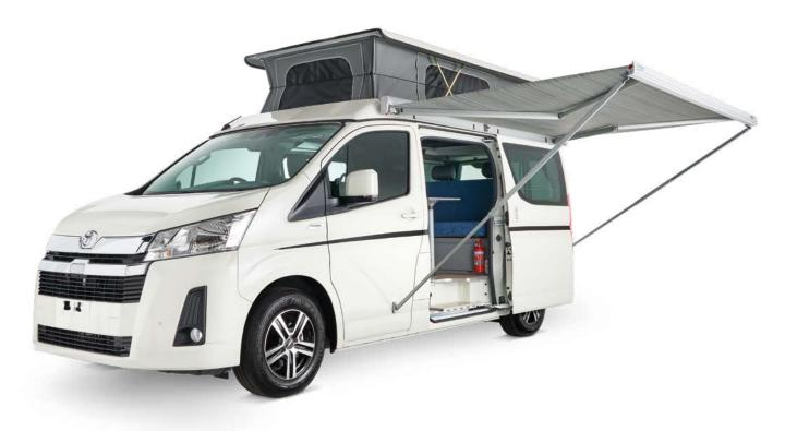
A significant development is the bonneted body style that places the engine up front, providing increased front end collision protection. Being seated behind the engine bay, allows for comfortable bucket seats for increased comfort, plus a walk-through cabin for increased functionality. With further improvements to safety, the HiAce now includes seven airbags and obtains a 5-star ANCAP rating.
