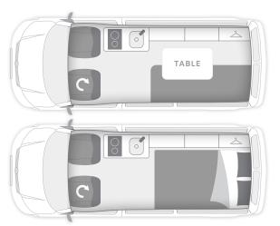
SEAT CONVERTS TO DOUBLE BED OR CAN BE BUILT WITH PERMANENT SINGLE BED.
